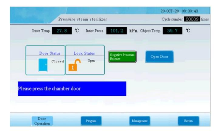
After the prompt "please press the chamber door" disappears, the hand can leave the cavity door, and the prompt interface is as follows:
