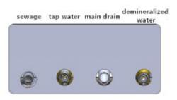
shown in the right figure of tap water), the main discharge branch (main drain) of booster pump inlet branch (as shown in the right figure of demineral water mark) and the evaporator drainage branch (sewage) marks. The distance between the equipment drain outlet and the connecting pipe of drainage pipe shall not be more than 0.5m, and the drainage pipe shall not have reverse pressure.
